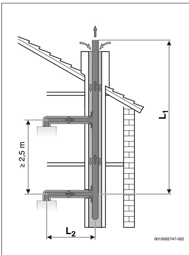
Fig. 22 Configuration C<sub>43p</sub>
