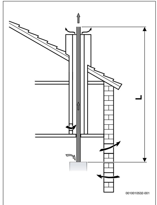
Fig. 15 Configuration B<sub>23p</sub> verticale
